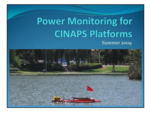
The research internship that I did at USC was centered around one of the autonomous boats to be used for aquatic sampling. The boat itself is around 4-6 feet long. Navigation is achieved using a combination of a GPS, compass, and IMU. Obstacle avoidance was to be done using a mounted sonar. The 'intelligence' of the unit was an Intel Atom-based mini-itx computer. Three batteries are used – one for the electronics, one for the sonar, and one for the electric motor/rudder.
