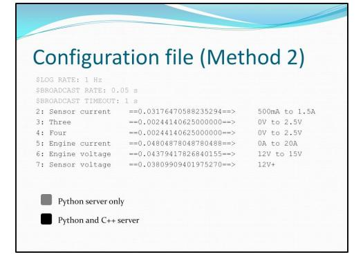
This is the configuration file used by the Overo server to convert the raw 10-bit ADC value to a floating-point current or voltage. The format is: Channel #: Name ==Calibration Multiplier==> minimum value to
