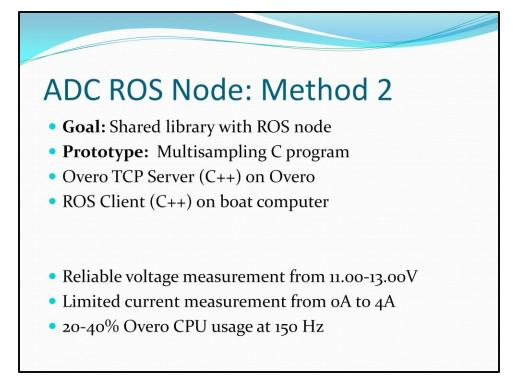
My second attempt was a big improvement. Rather than using an intermediate console program, the server got the data from the ADC directly using ioctl() calls. This allowed the server to sample-and-average the data and get accuracy comparable to the voltmeter I used to calibrate with. The current accuracy was not as impressive but was improved. Finally, I was able to use the same source code library to build the Overo server and the ROS client.
