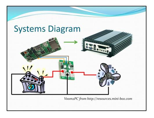
My primary project for the summer was to design a power monitor to determine how much power was being used by certain components. There also existed a sister project to the boats which used solar-powered monitoring buoys for taking measurements from stationary positions. A power monitoring system would also allow the buoys to report how much solar energy they were receiving and how charged their batteries were.
