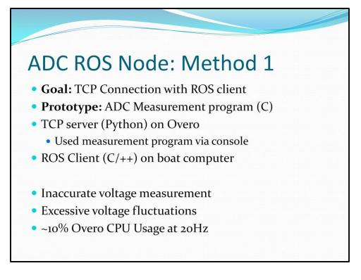
My first attempt used a Python server to read the ADC output from a console program and broadcast it to the boat's main computer. This approach was not very accurate, and seemed very inefficient to me since it required the Python server to start a process every time it took a measurement.
